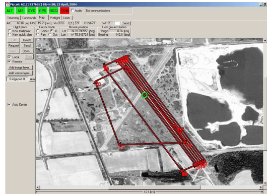
Fig. 6. Example single UAV search pattern at the Bridgeport Airport, New Jersey test site.
