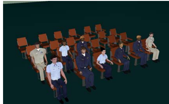
Figure 1: This diagram shows an image from the Human Modeling Software Testbed (HMST). This is an ergonomic test platform tool based on the Jack and Process Simulate Human toolkit. The tool allows users to test designs of new environments with virtual people and test many human factors, such as timing, efficiency, reachability, lines of sight, and user comfort.
