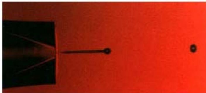
Figure 6.9 Demand mode ink-jet printing where only a small amount is needed with great accuracy 9 .
