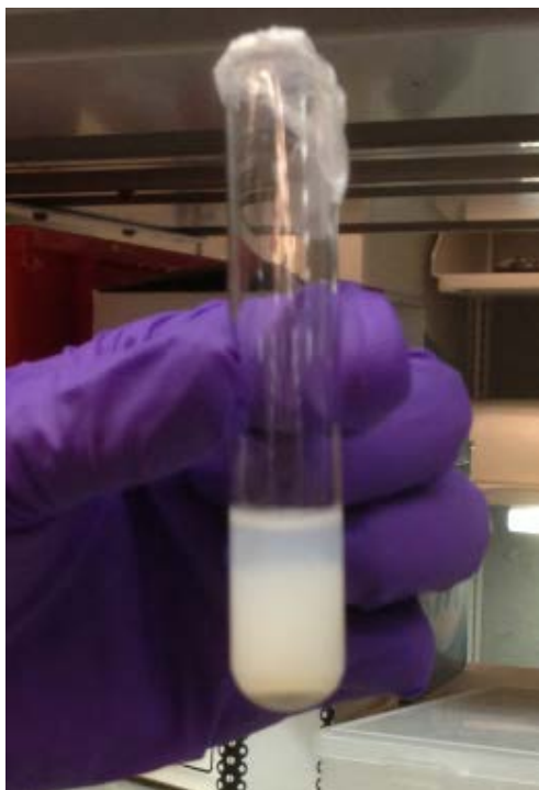
Figure 5.27: Kaolin mixed with water, centrifuged briefly, and allowed to settle overnight. Three distinct bands appeared within the solution, with the heavier particles at the bottom. For the kaolin-collagen surface, the top layer was used.
