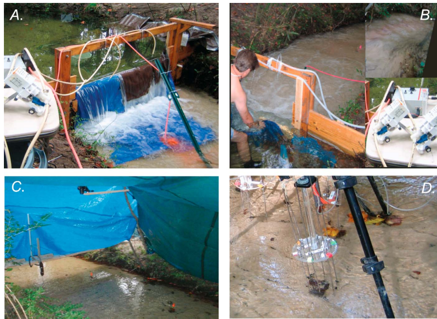
Figure 3. (a) Solute and fluorescent particulate tracers were injected into Clear Run for 3.5 h during a time period of steady base flow. (b) One hour after the injections ceased a small flood was created by releasing water through the dam. Before and after the flood, (c) time-lapse photo imaging of bedform migration was conducted using a tripod mounted camera that had been programmed to shoot on 30 s intervals as well as (d) in situ sampling of solute and fine particulate tracer breakthrough at shallow depths in the streambed using the USGS MINIPPOINT sampler.
