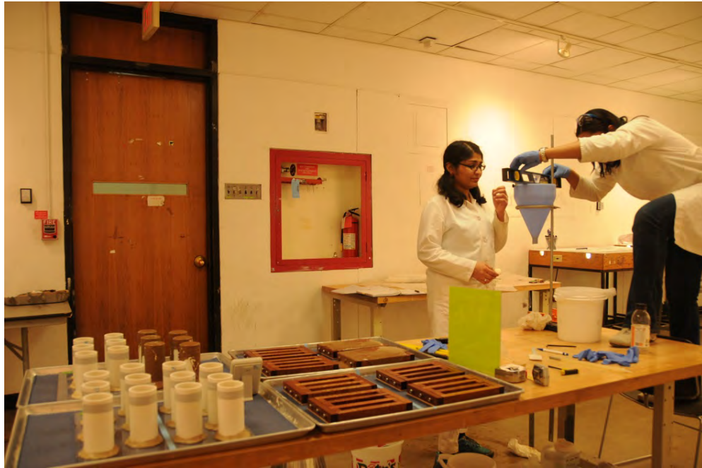
Figure 43: Leveling the flow cone before performing the flow test Source: Iyer 2014 (Setup a tripod)
