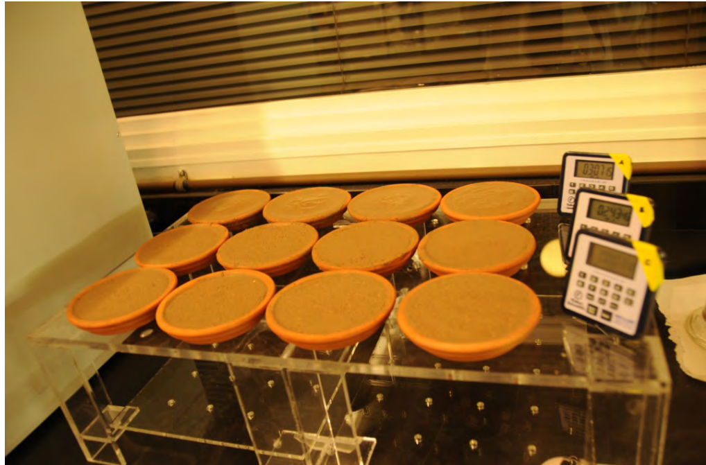
Figure 41: All test samples poured into unglazed terracotta saucers (Day 1) Source: Iyer 2014
