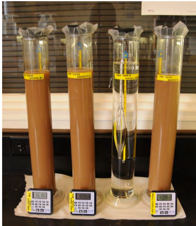
Figure 31: Soil samples and control in cylinder Source: Iyer 2014
