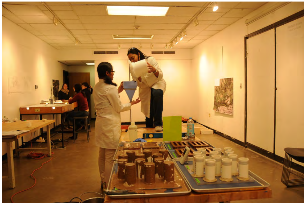
Figure 44: Pouring the measured grout sample for the flow test Source: Iyer 2014 (Setup a tripod)
