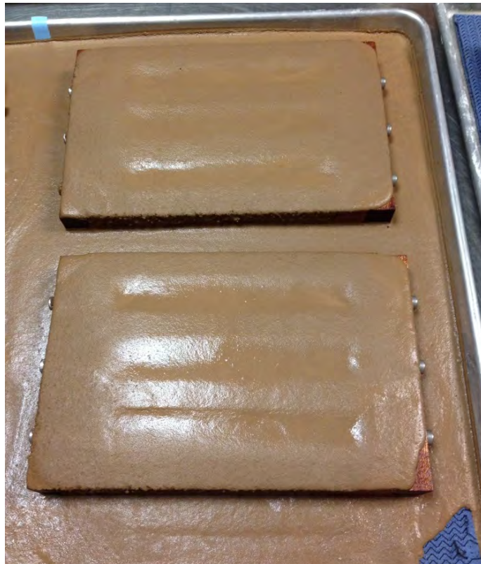
Figure 52: Drying shrinkage prisms for Sample B Source: Iyer 2014
