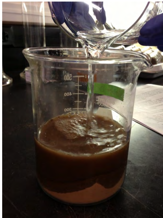
Figure 23: Adding 4% solution of sodium hexametaphosphate to soil sample Source: Iyer 2014
