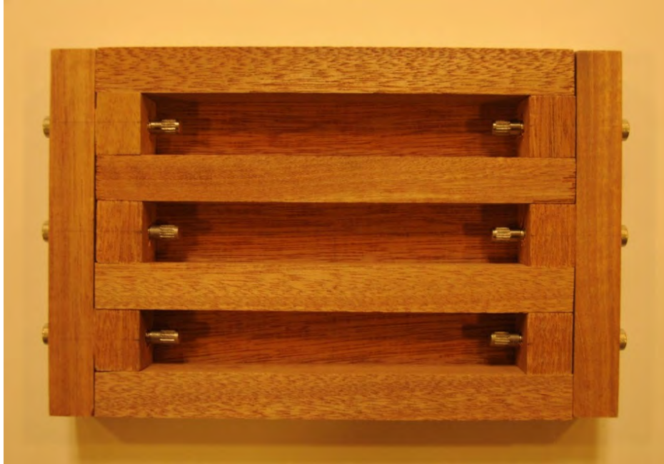
Figure 7: Custom made drying shrinkage prisms Source: Iyer 2014
