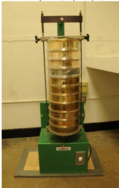
Figure 22: Mechanical shaker used to execute the sieving process Source: Iyer 2014
