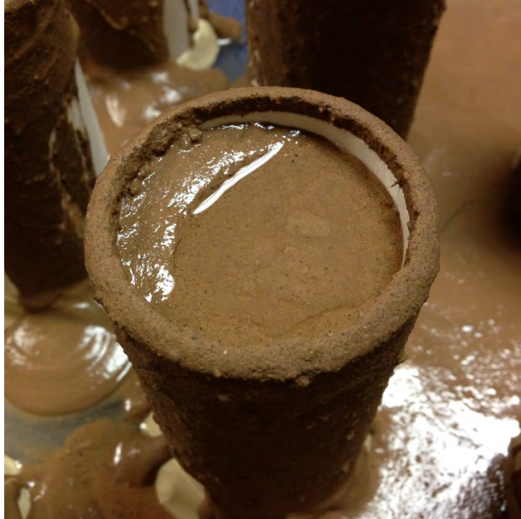
Figure 48: Separation of water from the grout sample observed (Sample A) Source: Iyer 2014
