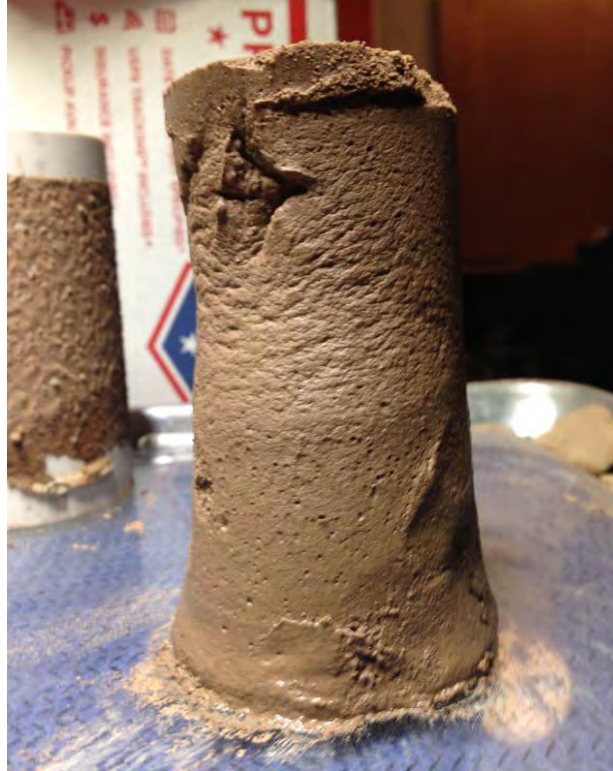
Figure 16: Sample B deformed during demolding Source: Iyer 2014
