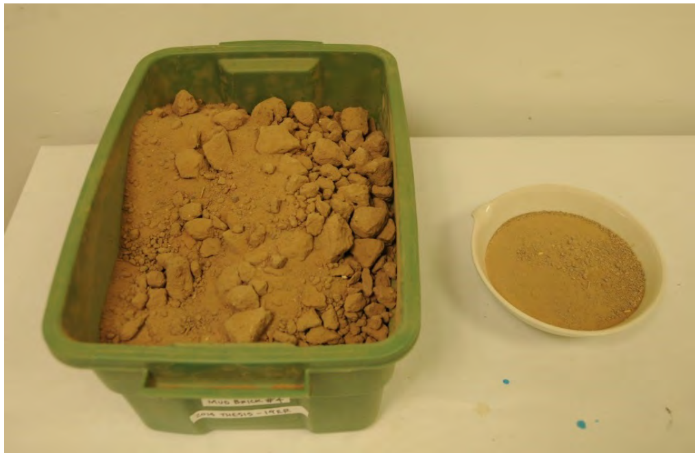
Figure 3: Mechanical crushing mud bricks Source: Iyer 2014
