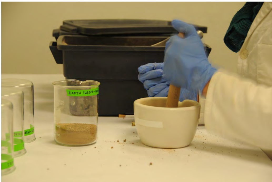
Figure 4: Using Mortar and Pestle to crush the sample Source: Iyer 2014
