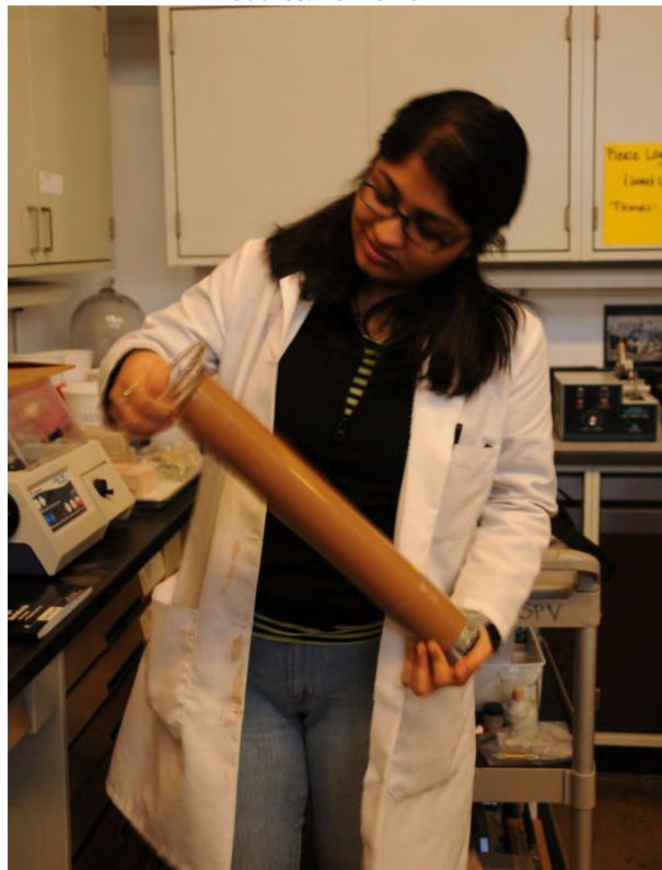
Figure 30: Agitating cylinder prior to starting sedimentation experiment Source: Naima 2014
