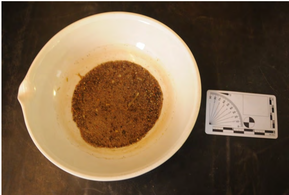
Figure 27: Sample get to dry in evaporating dish before placing in oven Source: Iyer 2014
