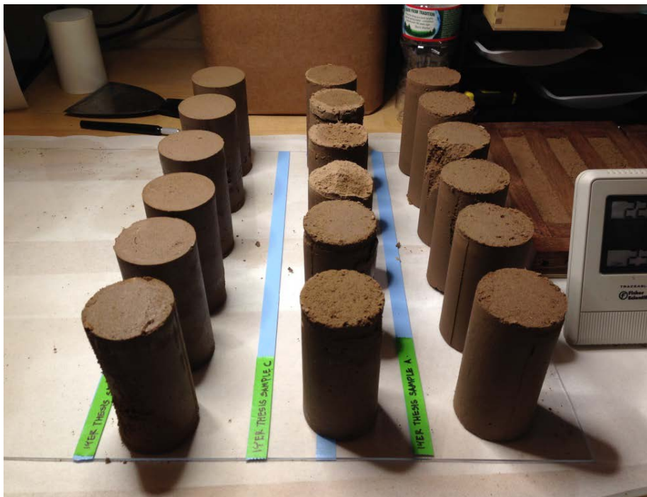
Figure 15: Splitting tensile samples left to cure (after demolding) Source: Iyer 2014
