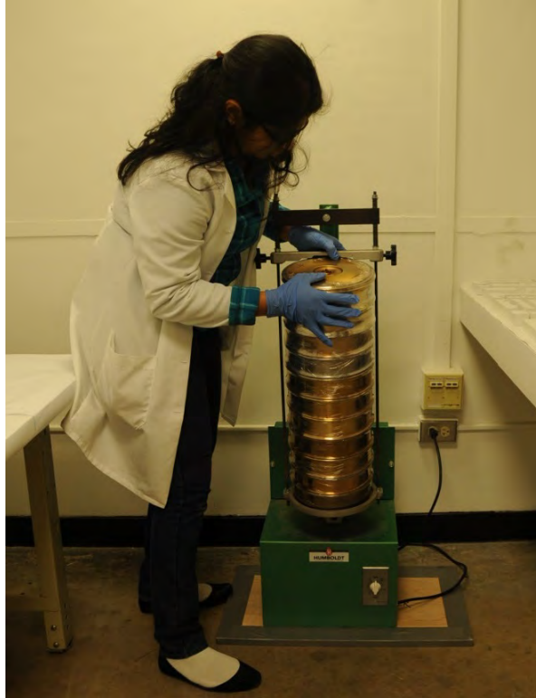
Figure 21: Securely placing the sieve stack on the mechanical shaker Source: Iyer 2014 (Setup the tripod)
