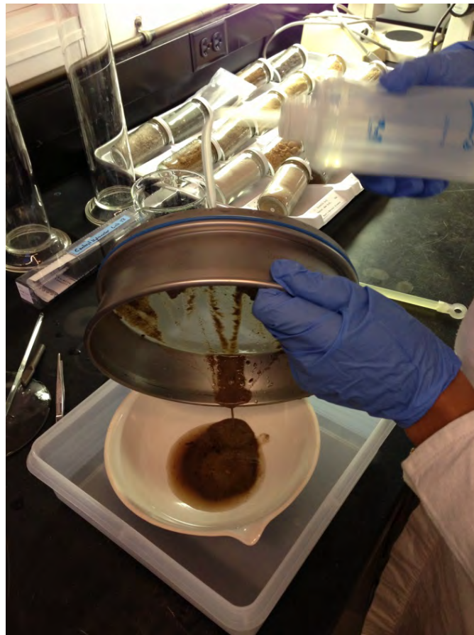
Figure 26: Collecting coarse particles by backwashing Source: Naima 2014
