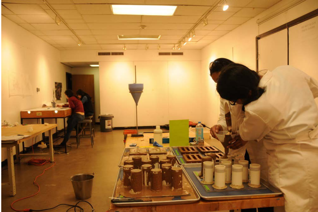
Figure 11: Pouring grout formulations into molds Source: Iyer 2014 (Set on tripod)
