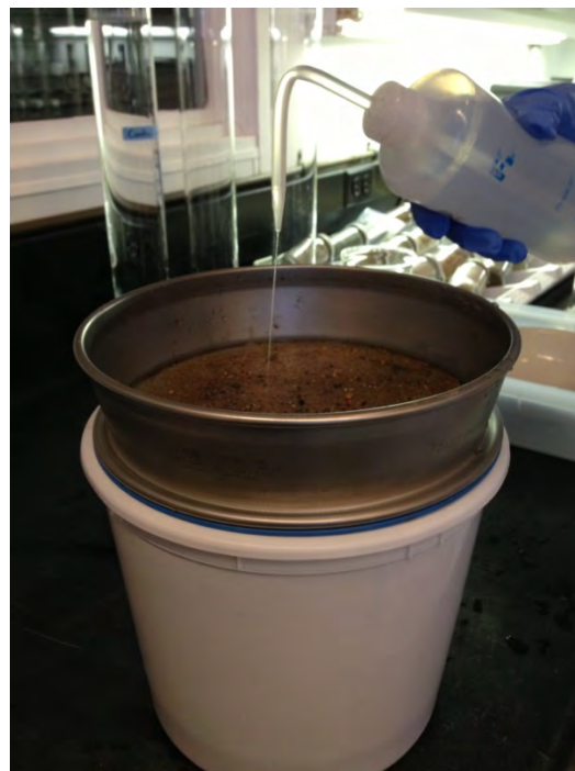
Figure 25: Separating fine soil particles by wet sieving Source: Naima 2014
