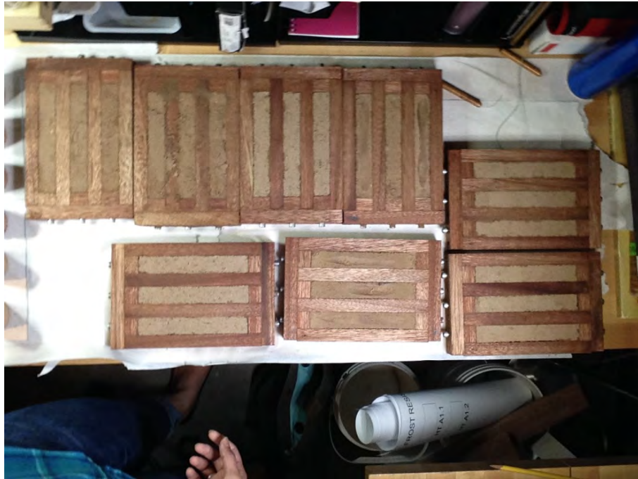
Figure 14: Drying shrinkage prism samples left to cure Source: Iyer 2014
