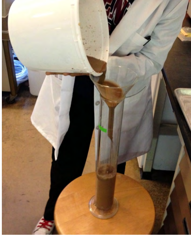
Figure 29: Transferring fine particles into sedimentation cylinder Source: Naima 2014
