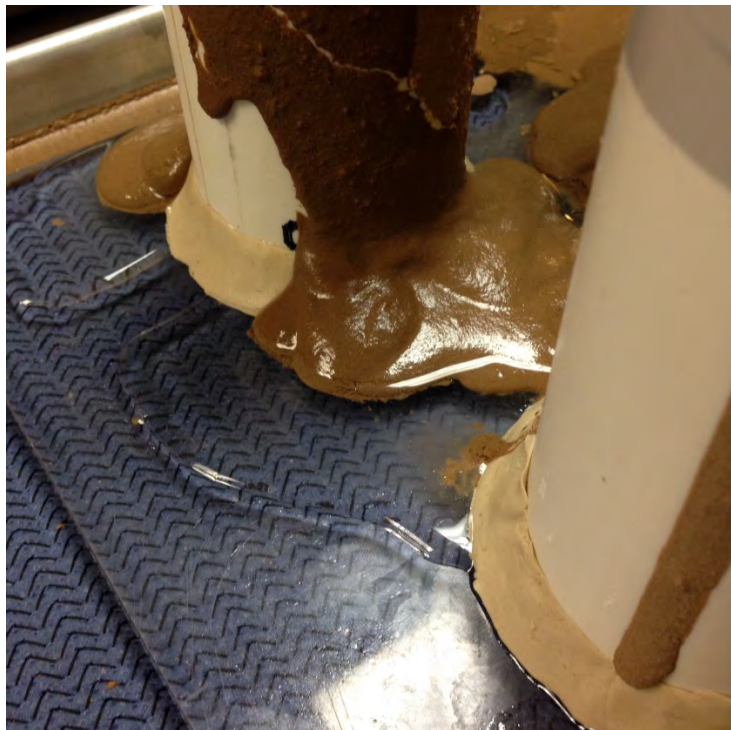
Figure 49: Clear water observed close to the plumber's putty (Sample A) Source: Iyer 2014
