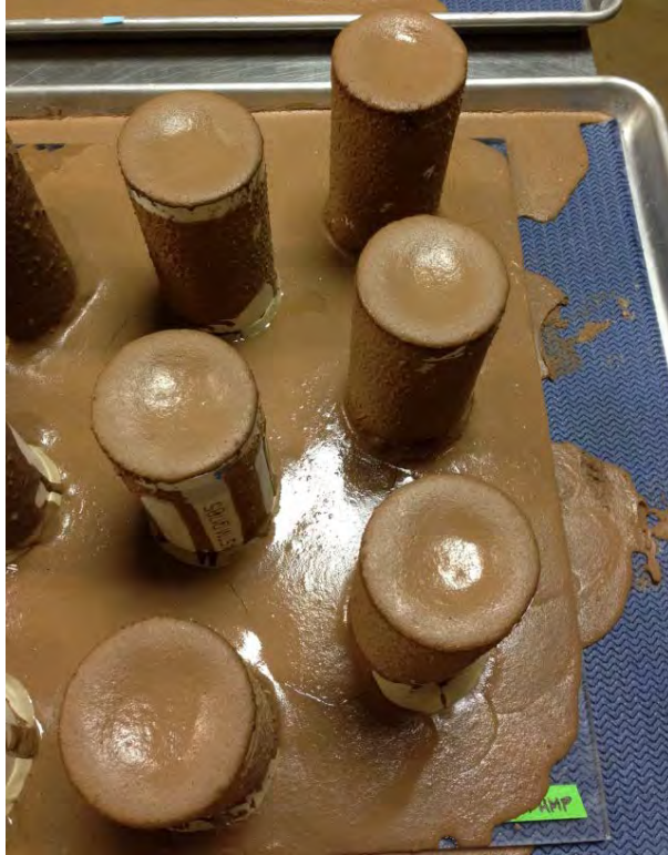
Figure 46: Splitting tensile samples for Sample B Source: Iyer 2014
