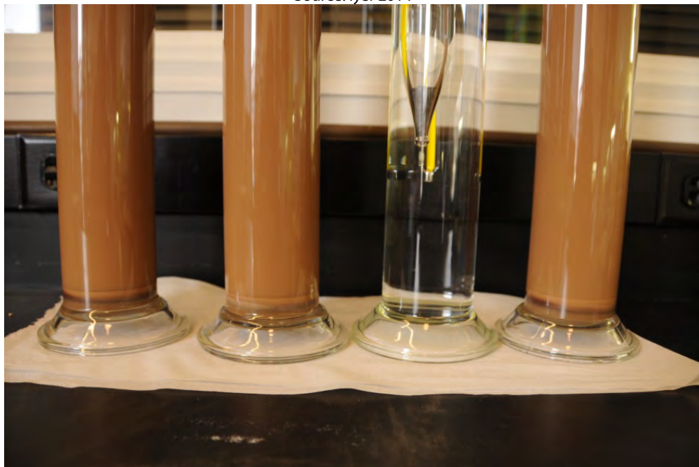
Figure 32: Detail of sedimentation observed in soil samples and control cylinder Source: Iyer 2014
