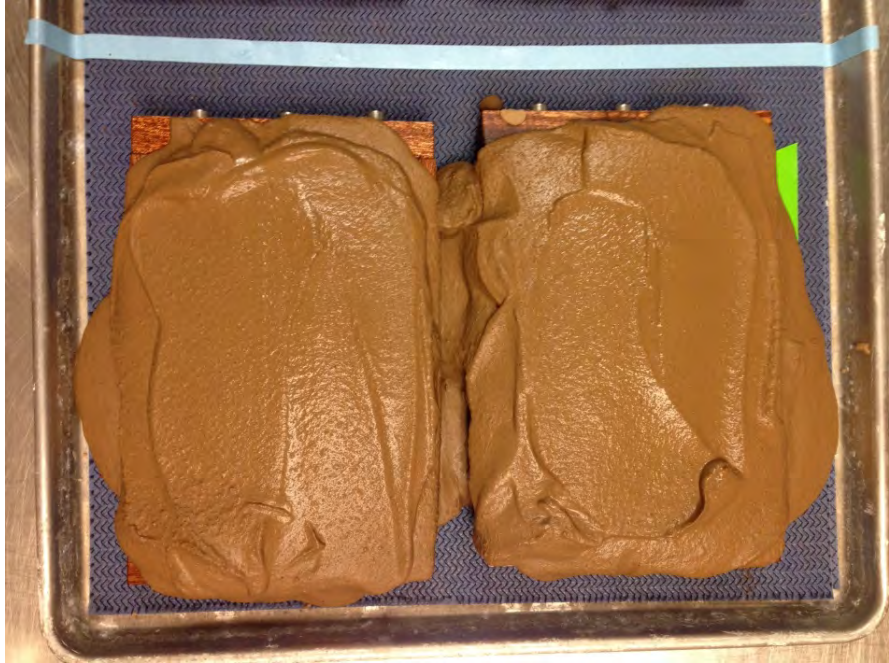
Figure 51: Drying shrinkage prisms for Sample C Source: Iyer 2014
