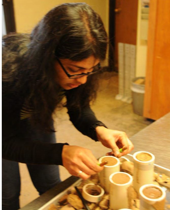
Figure 12: Using wire clay cutter to shape samples while demolding Source: Naima 2014
