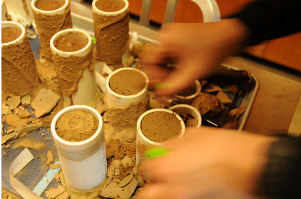
Figure 13: Detail shot of shaping samples while demolding Source: Naima 2014
