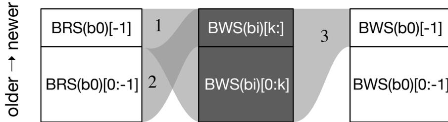
**Figure 6.7: Curd-Eager inter-block race checks involve three set intersections between each distinct pair of blocks. This example illustrates the checks between blocks  $b_0$  and  $b_i$ .**
