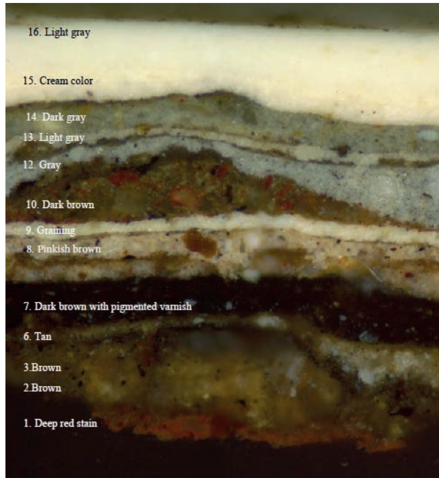
Figure G: Stratigraphy from original baseboard, trapped behind modern baseboard in Nathaniel Russell's Laundry 41
