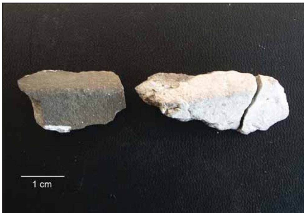
Figure 4.3: Limestone sample with black encrustation compared to sample cleaned with ion exchange resin (Source: Martínez-Arkarazo, 515).
