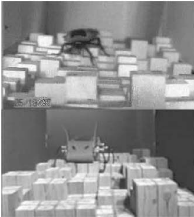
Fig. 2. Comparative views of locomotion in the rough: the cockroach Blaberus discoidalis (top photo, courtesy of R. J. Full) runs at 3.7 body lengths ( \sim 24 cm) per second (Full et al. 1998), whereas RHex (bottom photo) presently runs at only one body length ( \sim 50 cm) per second over comparably scaled broken terrain (see Extensions 3 and 4 ).
