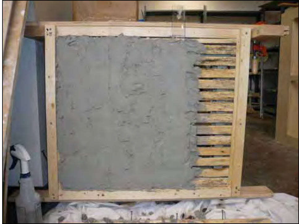
Figure 17: Plaster mock-up “B” – simulating detachment between the lath and the scratch coat.
