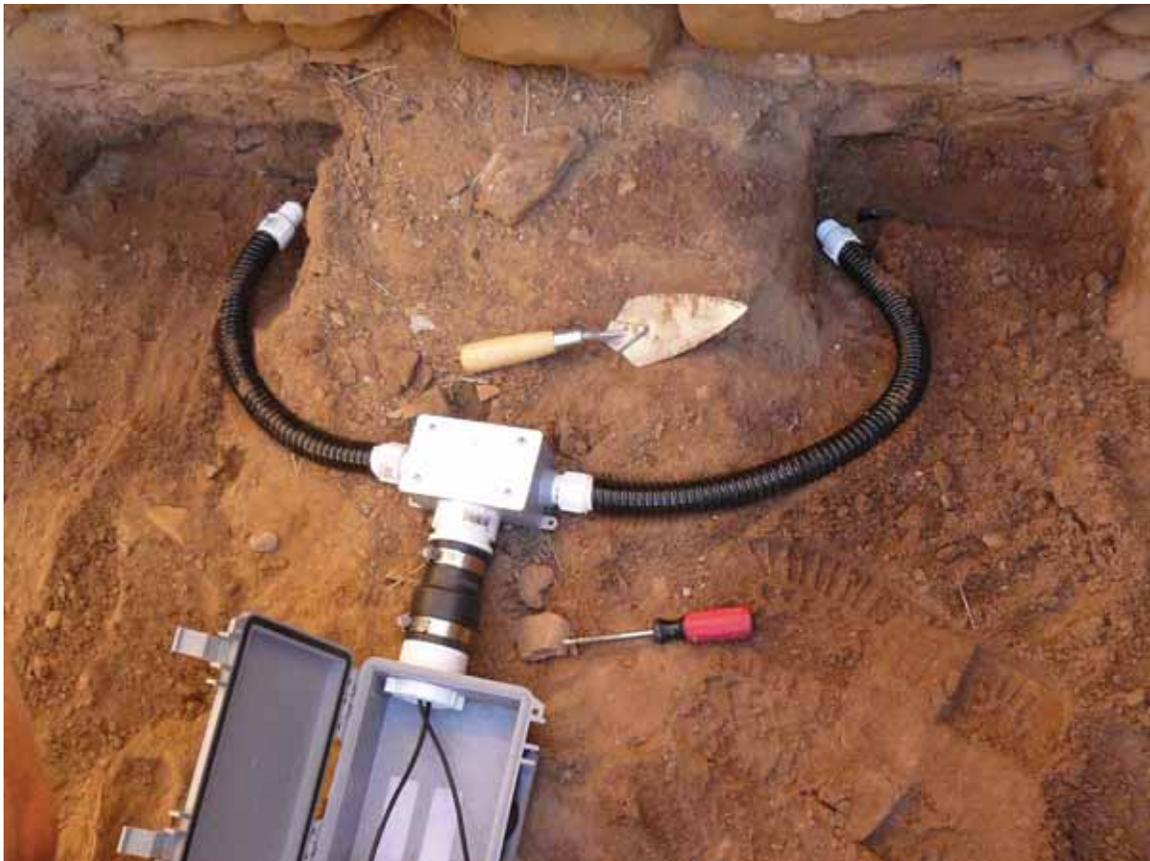
**Figure 30. Installation of Ground Soil Moisture Probe (Lim 2008)**
