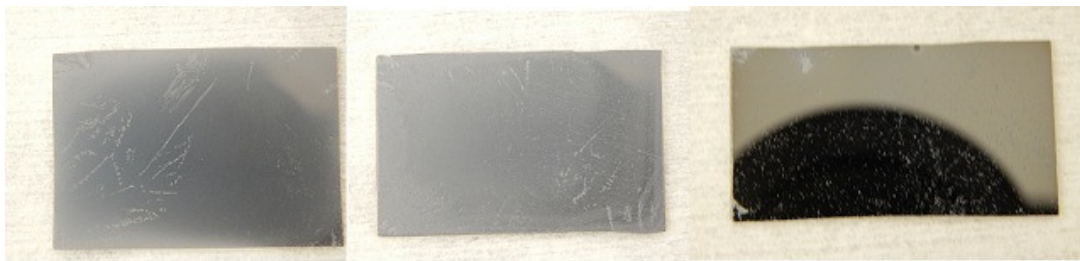
25 nm thick SiO2 on Si wafer
