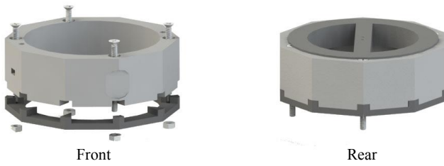
Fig. 4. The end caps are composed of two pieces that clamp together to hold the origami skin. Left: Front cap with pieces separated. The pieces are assembled using four M3 screws (35 mm in length) and nuts. Right: The rear end cap (assembled), which serves as the nozzle, also has a cross-bar for attaching the fishing line.
