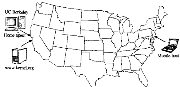
Fig. 11. The autonomous HA placement decision made by DHARMA. Notice how this allows the MH almost unrestricted movement without incurring additional routing overheads.
