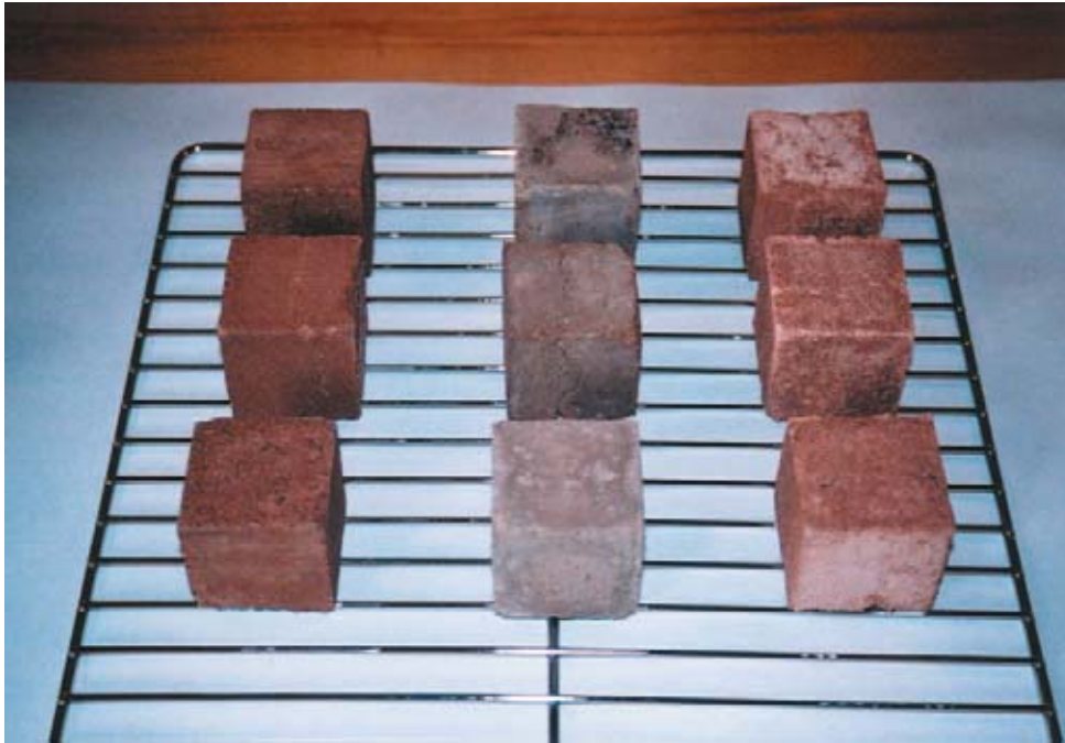
Figure G-1: The bedding mortar samples before first cycle of 14% solution of sodium sulphate decahydrate immersion and drying in oven. Left: Hydrated hydraulic lime. Center: Portland cement. Right: Lime putty.
