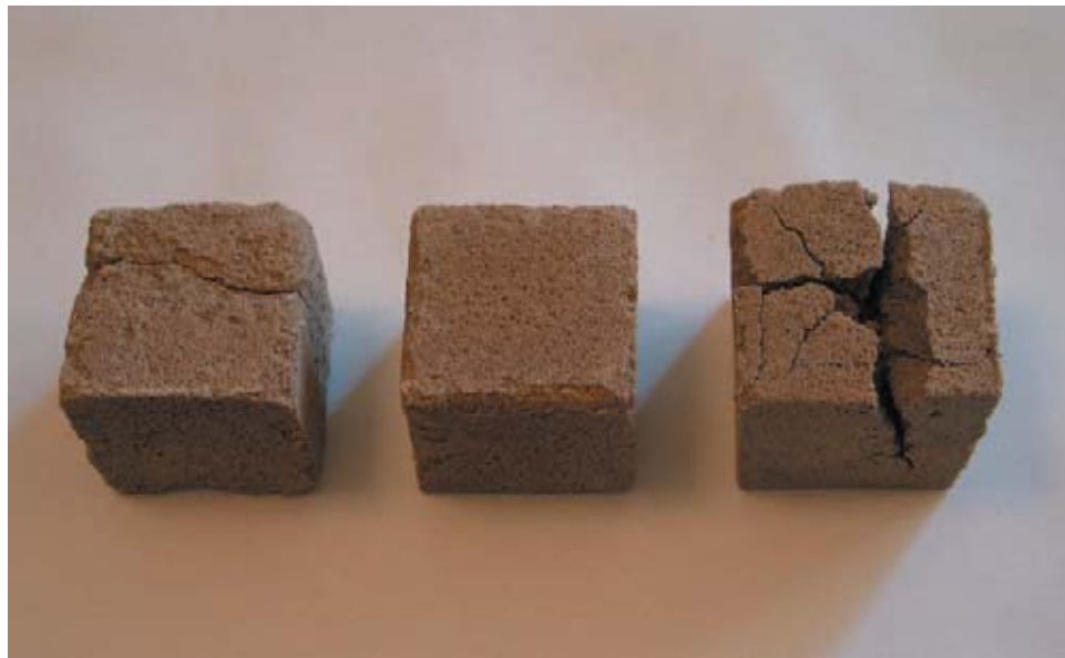
Figure G-6: The hydrated hydraulic lime finish pointing mortar samples after 15 cycles of immersion in 14% solution of sodium sulphate decahydrate immersion and drying in oven. Left: fh.1 Center: fh.2 Right: fh.3. Notice disaggregation at edges and cracking of fh.1 and fh.2 and fracture from internal stress of fh.3.
