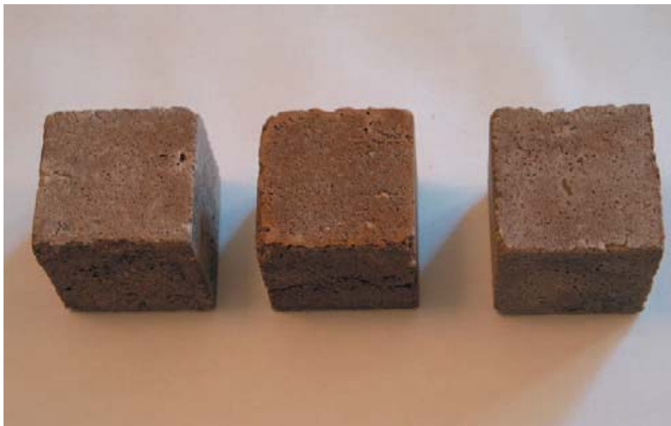
Figure G-4: The Portland cement bedding mortar samples after 15 cycles of immersion in 14% solution of sodium sulphate decahydrate immersion and drying in oven. Left: bc.1 Center: bc.2 Right: bc.3. No change occurred in shape or edges of bh.1 and bh.3., but bh.2 exhibits disaggregation at the corners. Please note, line on the side of sample bh.2 is original to sample.
