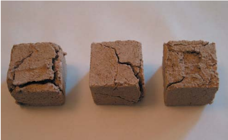
Figure G-8: The lime putty finish pointing mortar samples after 15 cycles of immersion in 14% solution of sodium sulphate decahydrate immersion and drying in oven. Left: fp.1 Center: fp.2 Right: fp.3. Notice fracture occurred in all samples.
