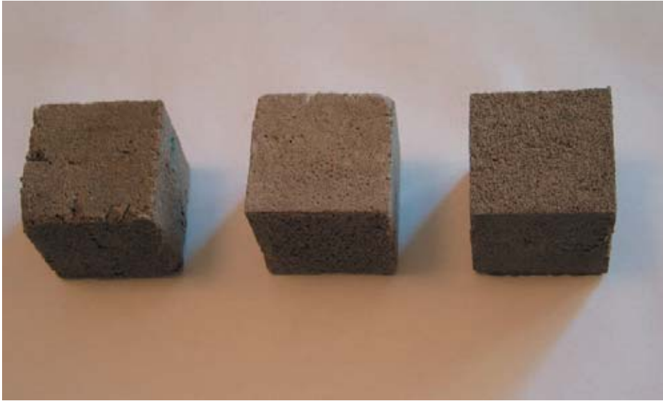
Figure G-7: The Portland cement finish pointing mortar samples after 15 cycles of immersion in 14% solution of sodium sulphate decahydrate immersion and drying in oven. Left: fc.1 Center: fc.2 Right: fc.3. No change in shape or edges and corners occurred (fc.1 inconsistencies original to sample).
