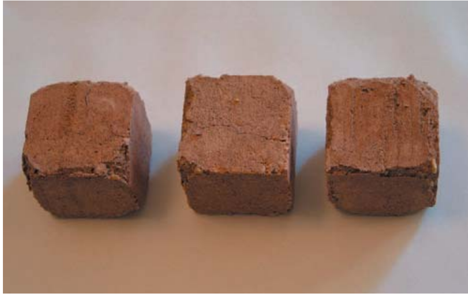
Figure G-5: The lime putty bedding mortar samples after 15 cycles of immersion in 14% solution of sodium sulphate decahydrate immersion and drying in oven. Left: bp.1 Center: bp.2 Right: bp.3. Notice disaggregation at edges and corners.
