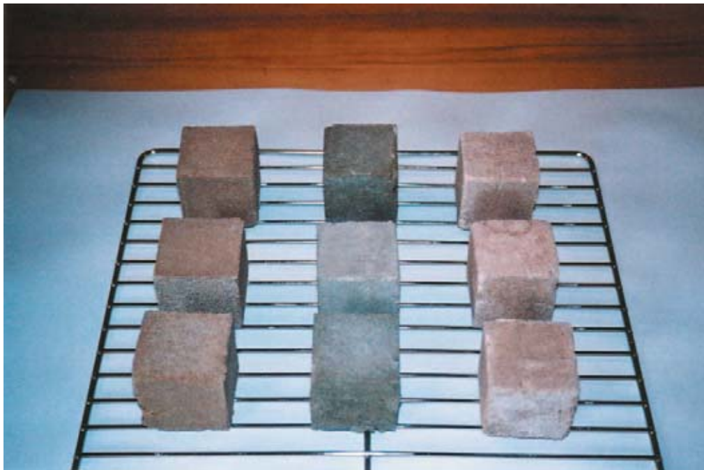
Figure G-2: The finish pointing mortar samples before first cycle of 14% solution of sodium sulphate decahydrate immersion and drying in oven. Left: Hydrated hydraulic lime. Center: Portland cement. Right: Lime putty.
