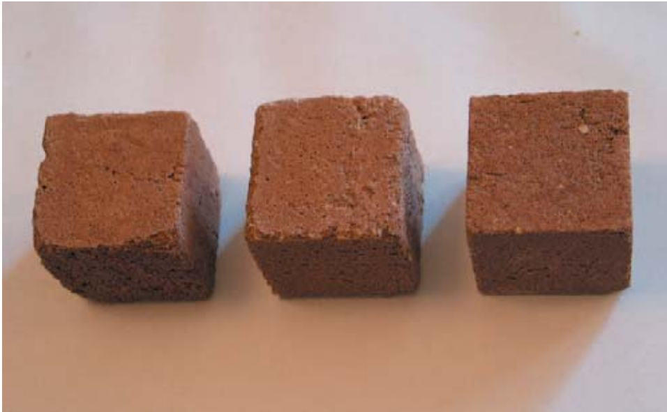
Figure G-3: The hydrated hydraulic lime bedding mortar samples after 15 cycles of immersion in 14% solution of sodium sulphate decahydrate immersion and drying in oven. Left: bh.1 Center: bh.2 Right: bh.3. Notice disaggregation at corners and edges of bh.1 and bh.2.
