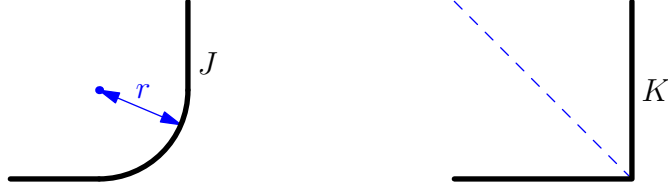
Figure 6.4: The set J has reach r (the radius of the curve) since every point within r of J has a unique orthogonal projection onto J . The set K has reach 0 because points arbitrarily close to K (on the blue dotted line) have no unique orthogonal projection onto K .
