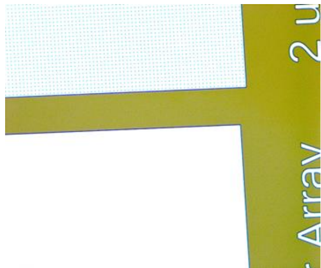
Figure 16: Absence of 1 μm pillar array, with 2 μm array for comparison (consistent feature across all wafers)
