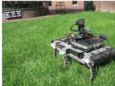
Fig. 1. Our experimental apparatus with XRHex [12] and visual fiducials [6] as a landmark (Section III) using the proposed controller (Section II) to move to a goal location while avoiding visual obstacles.
