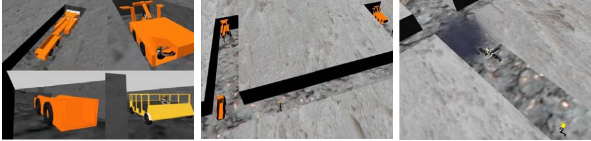
Figure 1: From left to right: (A) Coal mine equipment models; (B) Simulation of a normal working shift; (C) Simulation results on evacuation as smoke begins to envelop the miners
