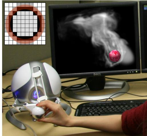
**Figure 1:** The user grasps the handle of the Novint Falcon to move the spherical object and feel the forces it experiences in the fluid. The inset shows a sample labeling of cells in the sphere’s vicinity, where light gray, black, dark gray, and white represent inside, boundary, surrounding, and outside cells respectively.
