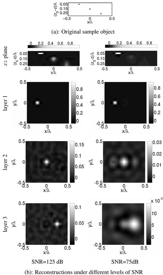
FIG. 2. Reconstructed images in vNFOT. (a) The sample. (b) Reconstructions in the  $xz$  plane and three transverse layers parallel to the  $xy$  plane in which the three point scatterers are located. Each image is normalized to its own maximum.
