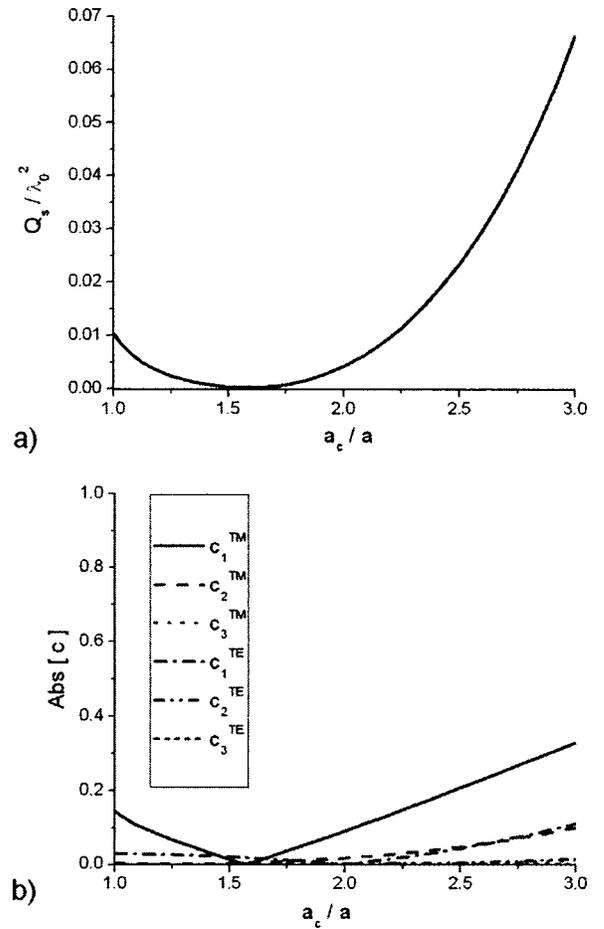
FIG. 7. (a) Normalized total scattering cross section and (b) contributions of the several (nonzero) scattering coefficients, in terms of the cover radius for a fixed inner core ( $\epsilon = 10\epsilon_0$ ,  $\epsilon_c = 0.5\epsilon_0$ ,  $\mu = \mu_c = \mu_0$ , and  $a = \lambda_0/10$ ).
