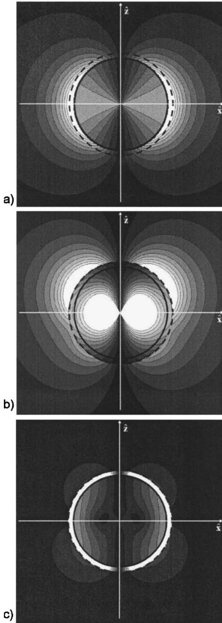
FIG. 13. Contour plots of the distribution of the radial components of the scattered electric field in the  $x$ - $z$  plane, induced by a plane wave traveling along the  $z$  axis with an electric field polarized along the  $x$  axis: (a) for a sphere with  $\epsilon=10\epsilon_0$ ,  $\mu=\mu_0$ , and  $a=\lambda_0/20$ ; (b) for the same sphere, but covered with  $\epsilon_c=5\epsilon_0$ ,  $\mu_c=\mu_0$ , and  $a_c=1.09a$ ; (c) the same as (b), but with  $\epsilon_c=0.1\epsilon_0$ .
