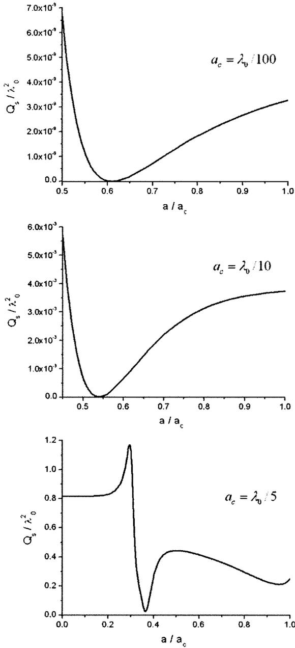
FIG. 3. Normalized scattering cross section for a spherical particle with  $\epsilon=4\epsilon_0$ ,  $\mu=\mu_0$ , and the cover with  $\epsilon_c=-3\epsilon_0$ ,  $\mu_c=\mu_0$ , versus the ratio  $a/a_c$  for three different sizes of the outer radius of the cover.
