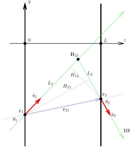
FIG. 1. (Color online) Illustrating the geometrical quantities used in Eq. (13). BR denotes broken ray.
