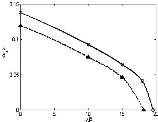
FIG. 10. The cross-sectionally averaged velocity  $\langle u_x \rangle$  is depicted as a function of the adverse pressure difference when the potential differences  $\Delta V=0.2$  V (dashed line with symbols ▲) and  $\Delta V=0.4$  V (solid line with symbols ○) are applied across the electrodes in the case of a single electrode pair ( $-5 \leq x \leq 5$ ,  $y = \pm 0.5$ ).  $C_0=0.1M$ ,  $H=1$  mm,  $L_E=10H$ , and  $L=30H$ .
