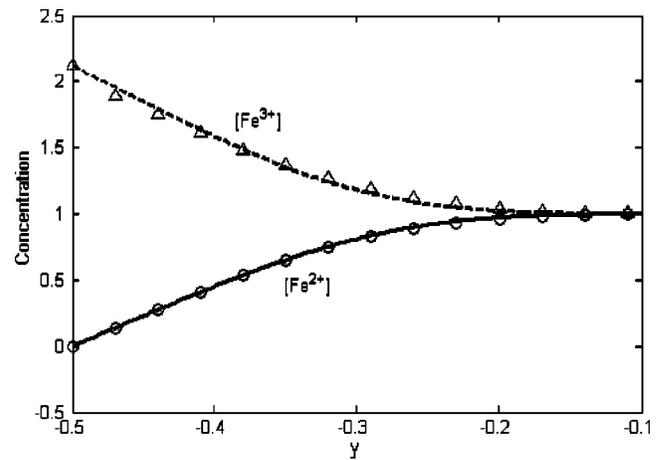
FIG. 12. The concentration distributions of the active ions  $\text{Fe}^{3+}$  (dashed line and  $\Delta$ ) and  $\text{Fe}^{2+}$  (solid line and  $\circ$ ) as functions of  $y$  at cross section  $x=0$  in the presence of abundant supporting electrolyte and under limiting current conditions in the case of a single electrode pair. The lines and symbols correspond, respectively, to the analytic boundary layer approximations and the numerical simulation.
