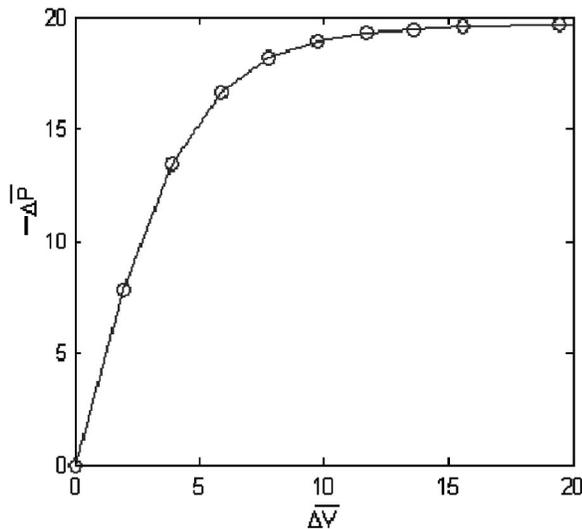
FIG. 11. The stall adverse pressure difference as a function of the imposed potential difference across the electrodes in the case of a single electrode pair ( $-5 \leq x \leq 5$ ,  $y = \pm 0.5$ ).  $C_0 = 0.1M$ ,  $H = 1$  mm,  $L_E = 10H$ , and  $L = 30H$ .
