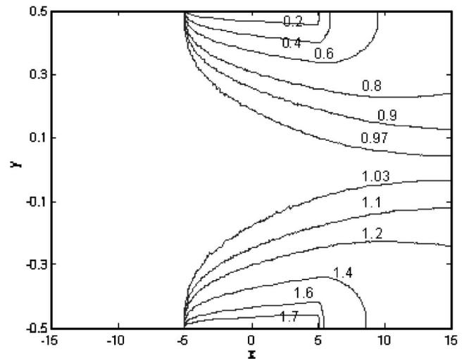
FIG. 2. The contours of the dimensionless concentration of the ion  $\text{Fe}^{3+}$  in a straight conduit with the electrode configuration depicted in Fig. 1(a). The imposed potentials on the surfaces of the anode ( $y = -0.5$  and  $-5 \leq x \leq 5$ ) and the cathode ( $y = 0.5$  and  $-5 \leq x \leq 5$ ) electrodes are, respectively,  $0.5 \text{ V}$  and  $-0.5 \text{ V}$ .  $\Delta \bar{p} = 0$ ,  $C_0 = 0.1M$ ,  $H = 1 \text{ mm}$ ,  $L_S/H = 10$ , and  $L/H = 30$ .
