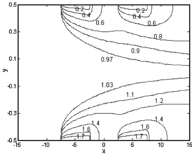
FIG. 3. The contours of the dimensionless concentration of the ion  $\text{Fe}^{3+}$  in a straight conduit equipped with two electrode pairs [Fig. 1(b)]. The imposed potentials on the surfaces of the anode ( $y=-0.5$ ,  $-7.5 \leq x \leq -2.5$ , and  $2.5 \leq x \leq 7.5$ ) and the cathode ( $y=0.5$ ,  $-7.5 \leq x \leq -2.5$ , and  $2.5 \leq x \leq 7.5$ ) electrodes are, respectively, 0.5 V and -0.5 V.  $\Delta\bar{p}=0$ ,  $C_0=0.1M$ ,  $H=1$  mm,  $L_E/H=5$ , and  $L/H=30$ .
