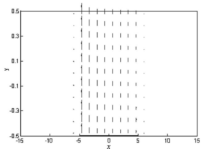
FIG. 5. The current flux field in a straight conduit. The imposed potentials on the surfaces of the anode ( $y=-0.5$  and  $-5 \leq x \leq 5$ ) and the cathode ( $y=0.5$  and  $-5 \leq x \leq 5$ ) electrodes are, respectively, 0.5 V and -0.5 V.  $\Delta\bar{p}=0$ ,  $C_0=0.1M$ ,  $H=1$  mm,  $L_S/H=10$ , and  $L/H=30$ .
