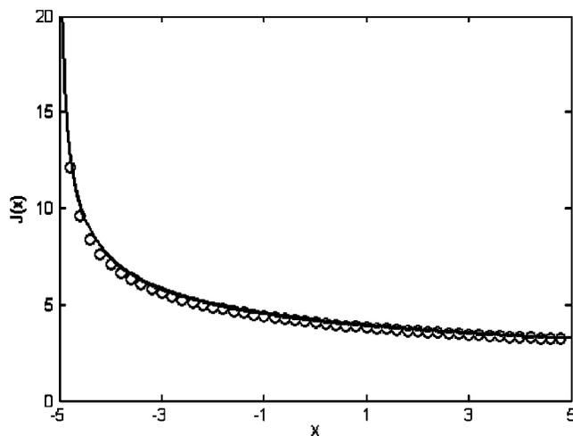
FIG. 13. The dimensionless limiting current flux as a function of  $x$  along the anode in the presence of abundant supporting electrolyte solution and under limiting current conditions in the case of a single electrode pair. The line and circles represent, respectively, the limiting current flux obtained with the analytic boundary layer approximation and the numerical simulation.
