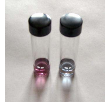
Figure 7. Colloidal gold solution before (left) and after (right) filtration through the microfluidic device.
