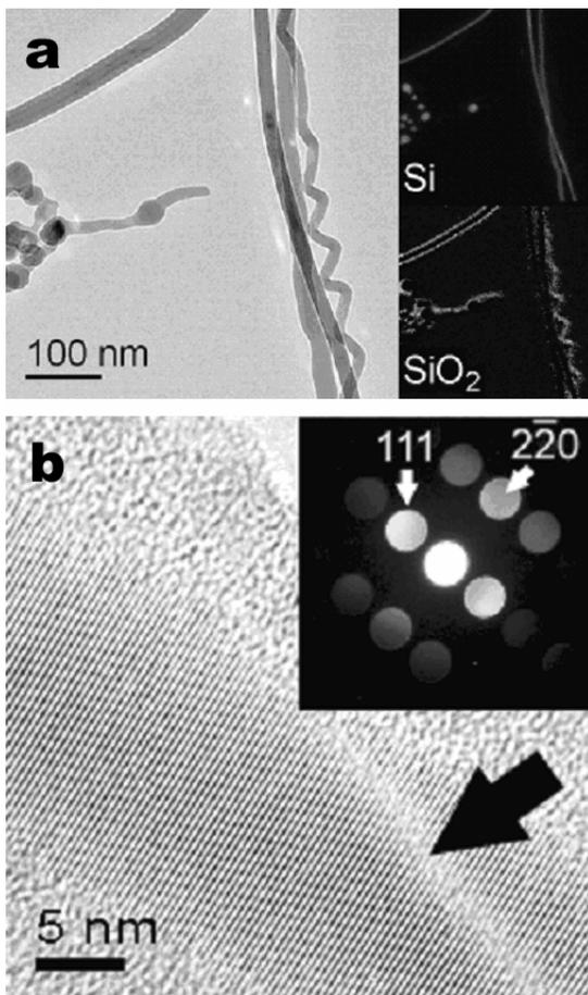
**FIG. 1.** (Color online) (a) EFTEM images were used to construct a color-coded map of the chemical environment of Si, where red represents crystalline Si, and green represents amorphous SiO<sub>2</sub>. (b) A high resolution TEM image of a SiNW grown along  $\langle 111 \rangle$ . The black arrow indicates the location of a stacking fault in the SiNW. Inset is the associated CBED pattern of the SiNW, taken along  $\langle 11\bar{2} \rangle$ . The (111) and  $(2\bar{2}0)$  disks are labeled.
