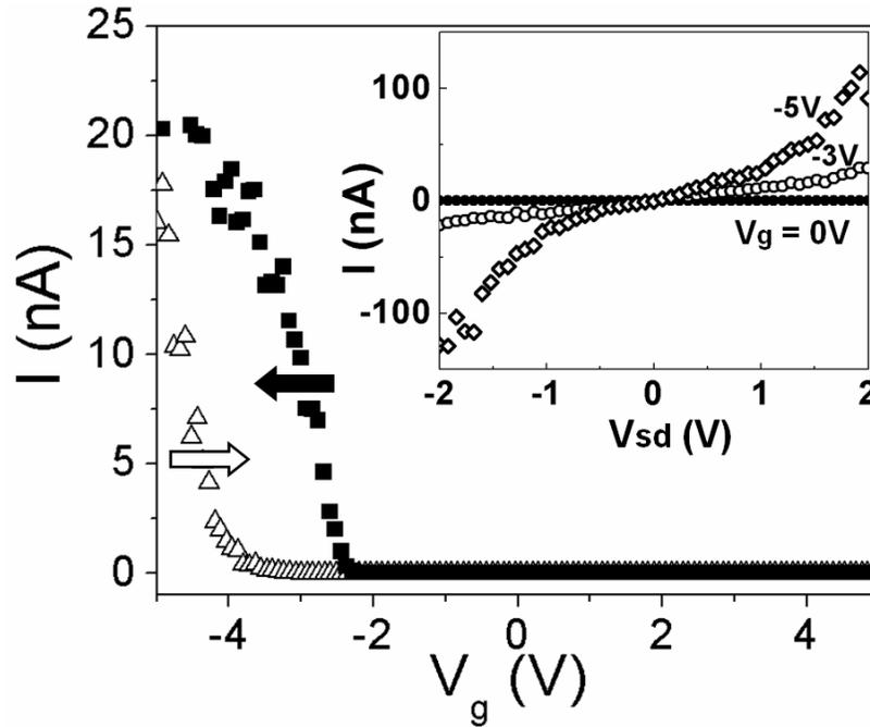
**FIG. 2.**  $I$ - $V_g$  data of an as-grown SiNW FET recorded for  $V_{sd} = 0.2$  V. The threshold voltages of the device depend on the gate sweep directions. Empty triangles represent the gate bias sweep from  $-5$  V to  $+5$  V while filled squares represent the gate bias sweep from  $+5$  V to  $-5$  V. (inset) a set of  $I$ - $V_{sd}$  data recorded at different gate voltages.
