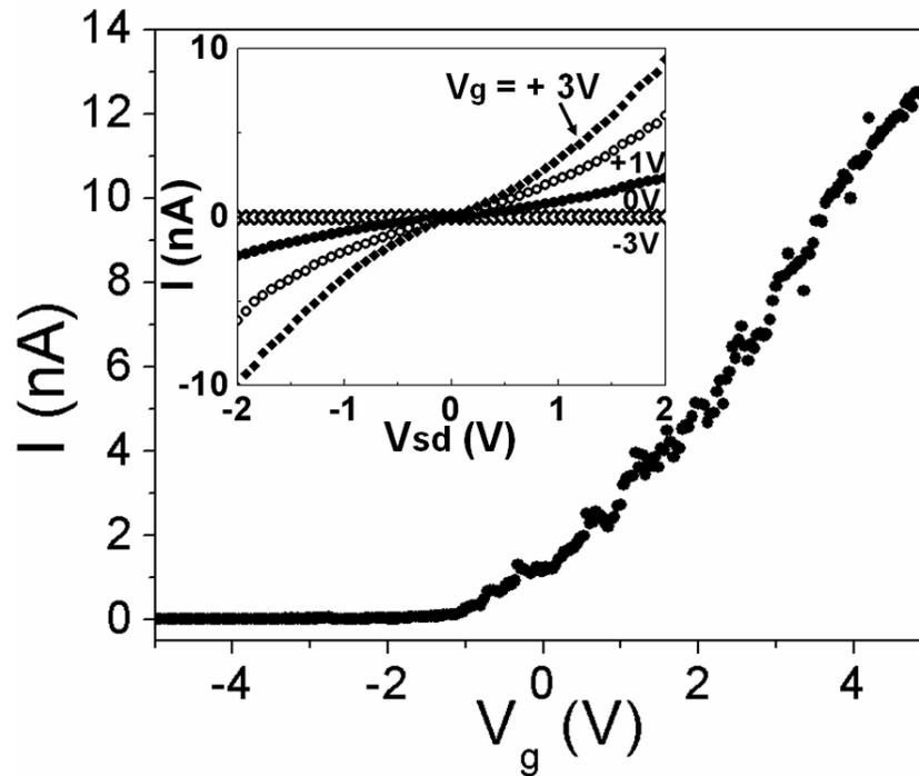
**FIG. 3.**  $I$ - $V_g$  characteristic of a Bi-doped SiNW FET recorded for  $V_{sd} = 2$  V. (inset) a set of  $I$ - $V_{sd}$  data recorded at different gate voltages.
