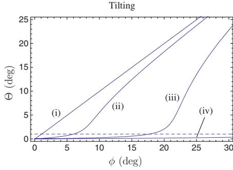
FIG. 5. (Color online) The tilt angle  $\Theta$  between the layer normal and the director as a function of the mechanical tilt angle  $\phi$  in the tilt apparatus for (i)  $\zeta/\mu=0.1$ , (ii)  $\zeta/\mu=1$ , (iii)  $\zeta/\mu=5$ , and (iv)  $\zeta/\mu=20$ . The dashed line corresponds to the resolution for  $\Theta$  in the experiments by KF.
