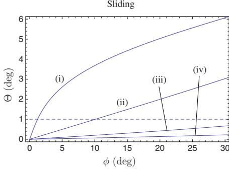
FIG. 3. (Color online) The tilt angle  $\Theta$  between the layer normal and the director as a function of the mechanical tilt angle  $\phi$  in the slider apparatus for (i)  $\zeta/\mu=0.1$ , (ii)  $\zeta/\mu=1$ , (iii)  $\zeta/\mu=5$ , and (iv)  $\zeta/\mu=20$ . The dashed line corresponds to the resolution for  $\Theta$  in the experiments by KF.
