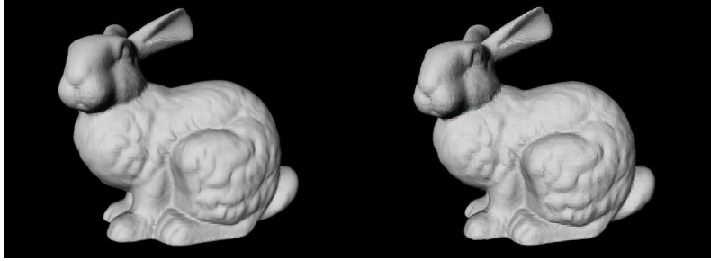
Figure 9: The original Stanford bunny model (left) and the output our algorithm at maximum octree level 7 (right).
