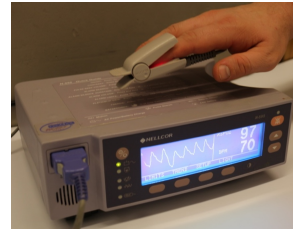
Figure 1: A pulse oximeter displaying a PPG waveform.
