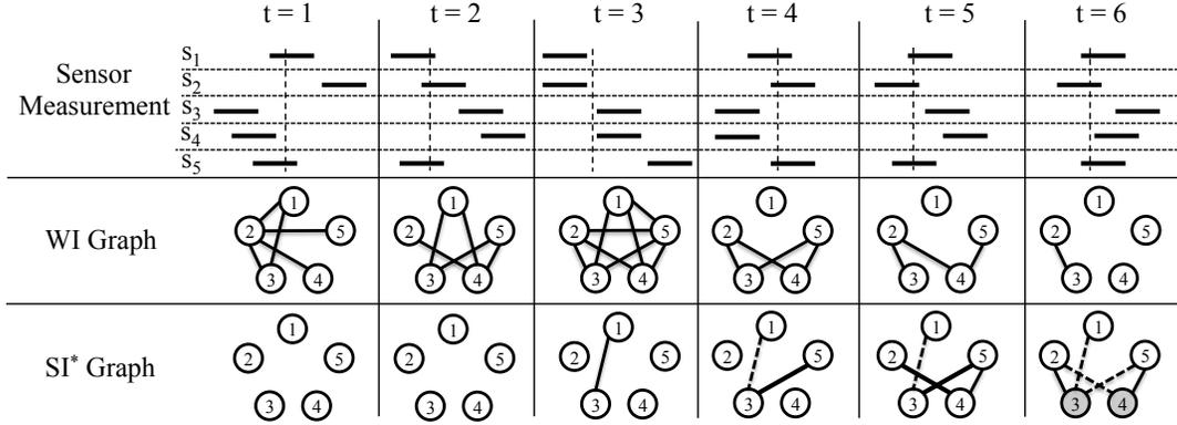
Figure 4: An example showing the detection and identification capabilities of the algorithm proposed in this paper. Dashed edges in the  $SI^*$  graphs indicated edges that were drawn in previous rounds.
