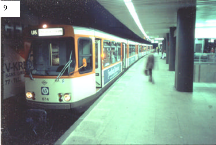
In city centers with congested streets, LRT typically uses tunnels (Frankfurt)
