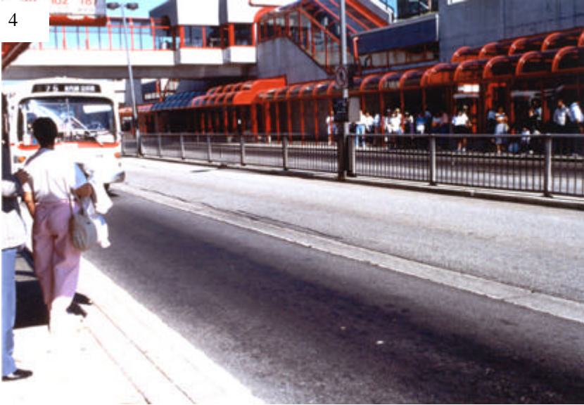
Fence in station prevents pedestrians from crossing the roadways (Ottawa)
