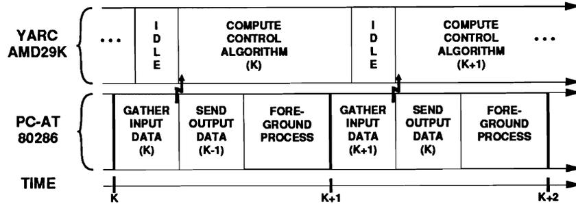
Figure 2: Timing Table of the Intel 80286 and AMD 29000
