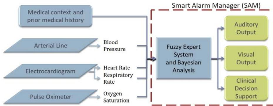
**Figure 1. Smart Alarms System Block Diagram**
