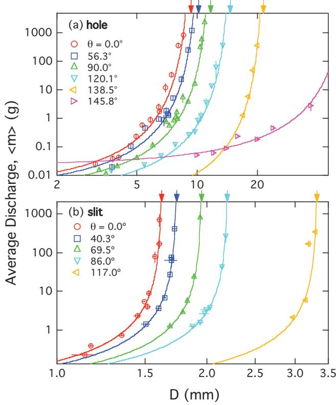
FIG. 6. (Color online) Average mass discharged versus aperture size  $D$  for glass spheres clogging in (a) circular holes and (b) long rectangular slits. Fits to the diverging power law of Eq. (3) are overlaid, with the exponents fixed to  $\gamma = 5$  for circular holes and 2 for rectangular slits, respectively. Critical aperture sizes from these fits are indicated by arrows.
