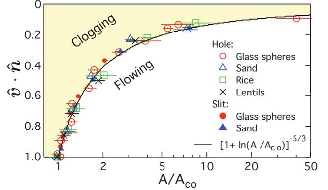
FIG. 10. (Color online) Clogging transition curves for most materials and *both* aperture geometries. The  $x$  axis is the hole area, normalized by the critical hole area at zero tilt angle. The  $y$  axis is the component  $\hat{v} \cdot \hat{n}$  of the average flow direction normal to the plane of the aperture (see Fig. 9 for illustration defining these unit vectors). The solid curve is an empirical fitting function; if allowed to float, the exponent is  $-1.84 \pm 0.02$ .
