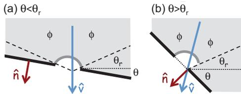
FIG. 9. (Color online) Geometry of the unit vectors  $\hat{n}$  and  $\hat{v}$ , specifying the normal to the plane of the aperture and the average flow direction, respectively, for cases that the tilt angle  $\theta$  is (a) less than, and (b) greater than, the angle of repose  $\theta_r$ . The average flow direction is defined by bisecting the region where the grains flow, i.e., so the two angles labeled  $\phi$  are equal.
