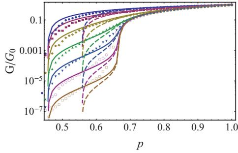
FIG. 9. (Color online) Comparison between the shear modulus (normalized by the shear modulus at  $p = 1$ , so it is equivalent to  $\mu_m/\mu$ ) obtained from numerical simulations from Ref. [35] (data points), Das's EMT (solid lines), and our EMT (dashed lines). Different colors mark different values of  $\kappa$  with the same color code as in Fig. 5, and from top to bottom the corresponding values of  $\kappa$  are  $1, 10^{-1}, 10^{-2}, \dots, 10^{-6}$ .
