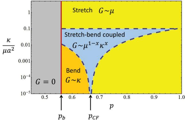
FIG. 1. (Color online) Phase diagram of the diluted filamentous triangular lattice showing the central-force and bending rigidity thresholds, respectively, at  $p = p_{CF}$  and  $p = p_b$ , the bending-dominated regime at small  $\kappa$  in the vicinity of  $p_b$ , the crossover bend-stretch regime near  $p_{CF}$ , and the stretching-dominated regime at large  $\kappa$ . (Adapted from Ref. [35].)
