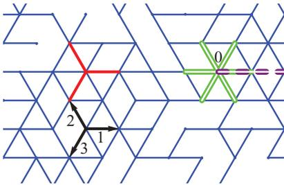
FIG. 3. (Color online) Filamentous triangular lattice with bonds randomly occupied with probability  $p$ . The unit vectors  $\mathbf{e}_1, \mathbf{e}_2, \mathbf{e}_3$  are marked by “1, 2, 3,” the 3 stretch energy vectors  $\mathbf{B}_n^s$  are marked by the 3 red single lines, and the 3 bending energy vectors  $\mathbf{B}_n^b$  are marked by the 3 green double lines. The purple dashed double line marks the bending vector  $\mathbf{B}_4^b$  if the origin is marked by 0.
