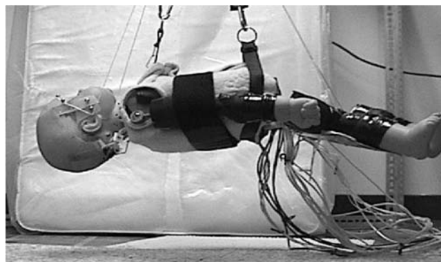
FIG. 5. Photograph representing a worst-case scenario. The surrogate was suspended and released in a supine position with legs extended and arms fixed to the torso. This configuration resulted in initial ground contact to occur with the head of the surrogate.
