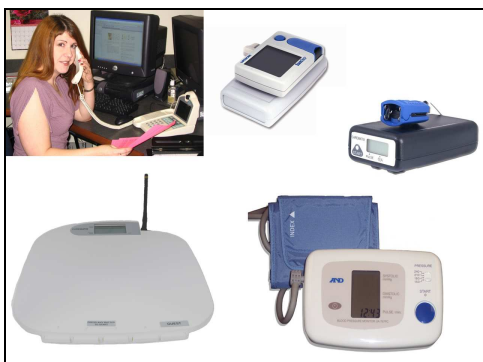
Figure 1. Telehealth equipment, nurse station, glucometer, pulse oximeter, blood pressure cuff, and scale (clockwise).
