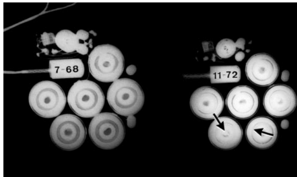
Fig 2. Radiographs of pacemaker in situ 15 months after implantation (left) and 5½ years after implantation (right). The radiolucent central cores and insulating rings between electrode cylinders in the batteries became filled by corrosion material (arrows) leading to battery failure.
