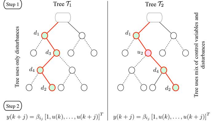
Fig. 1. Separation of variables. *Step 1:* Tree  $\mathcal{T}_1$  is trained only on the disturbances  $\mathcal{X}_d$  as the features. Tree  $\mathcal{T}_2$  uses both the disturbances  $\mathcal{X}_d$  and the control variables  $\mathcal{X}_c$  for splitting and is thus not computationally suitable for control. *Step 2:* In the leaf  $\ell_{i_j}$  of trees  $\mathcal{T}_j$ , a linear regression model parametrized by  $\beta_{i_j}$  is defined as a function only of the control variables.
