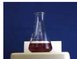
Figure 6. Photograph of a colloidal suspension of Au nanoparticles in water.
