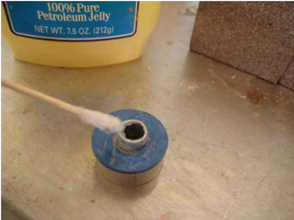
Figure 2.1. Injection Port and Fluorosilicone Washer. Photo by author
