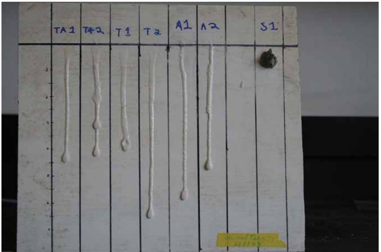
Figure 2.3 Flow tests with board upright. Photo by Author.
