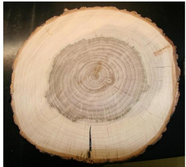
Figure 4, Cross section of catalpa.
