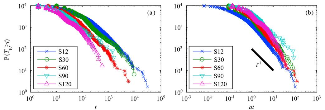
**Figure 4.** (a) Waiting time exceedance probability distributions ( $P(T_w > t)$ ) for the five experiments versus  $t$ . (b) Normalizing time by bed activity parameter,  $a$ , produces a reasonably good collapse of the data. Limiting power law scaling is slightly steeper than the  $t^{-1}$  line shown for comparison.
