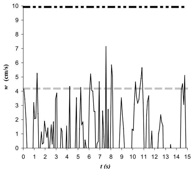
**Figure 11.** Upward directed instantaneous velocity,  $w$ , at  $z = 5 \times 10^{-3}$  m above the bed and  $x = 5.85$  m, measured for the rigid bed form case shown in Figure 10f. Also plotted are fall velocities,  $w_s$ , for medium (shaded dashed line) and coarse (solid dash-dotted line) sands.
