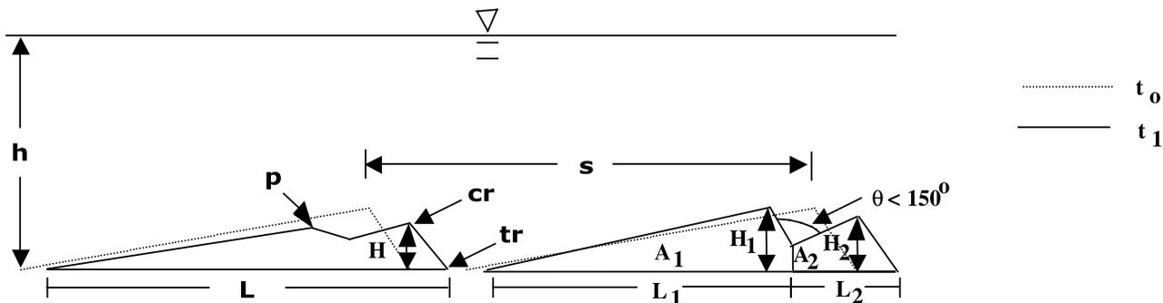
**Figure 2.** Definition sketch for experimental measurements. The bed form configuration is shown both at the beginning of an experiment ( $t_0$ ) and at some later time ( $t_1$ ). Bed form features include crest,  $cr$ ; trough,  $tr$ ; and peak (a local topographic high that is not a bed form crest),  $p$ .  $A_1$  and  $A_2$  are the cross-sectional areas associated with two separate bed forms originating from a single parent form. All other parameters are defined in the text.
