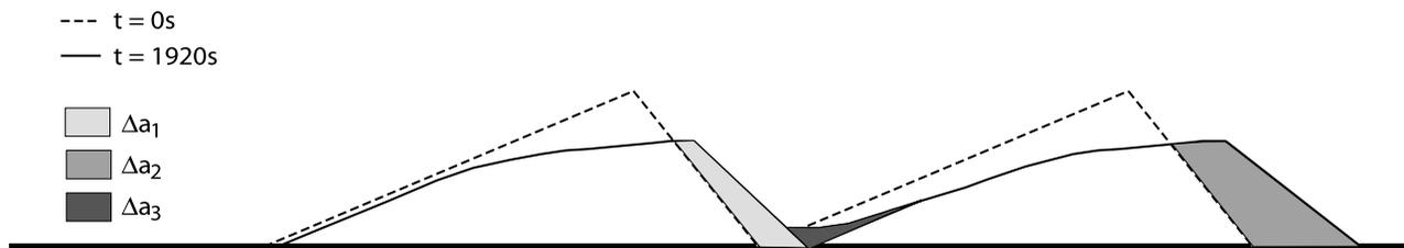
**Figure 4.** Changes in bed topography through time used to calculate local values for streamwise sediment discharge,  $q_s$  (equation (1)). The newly generated cross-sectional areas used to determine  $q_s$  at the crests of bed form 1 and bed form 2 are  $\Delta a_1$  and  $\Delta a_2$ , respectively. The cross-sectional area used to determine the upstream transport filling in the trough of bed form 1 is  $\Delta a_3$ .
