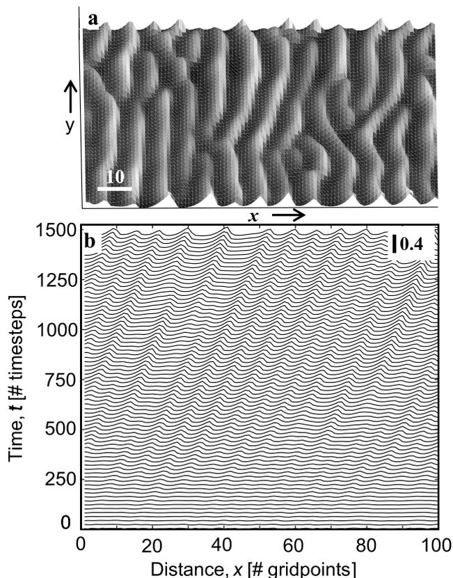
**Figure 4.** Deterministic model (run D, Table 1) evolution. (a) Oblique view snapshot of transient evolution of bed surface, at time =  $1500\Delta t$ . (b) Profile down the centerline of the 2-D model domain, showing growth of bed forms from a flat surface. Compare to Figure 4 of *Coleman and Melville* [1996]. Profiles are plotted every  $20\Delta t$  from zero up to time =  $1500\Delta t$ .
