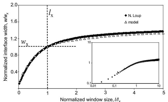
**Figure 7.** Example of spatial scaling of roughness for stochastic model (run S) and North Loup River at statistical steady state using a downstream profile at a snapshot in time;  $w$  and  $l$  are normalized by their transition values. See caption of Figure 2 for explanation; note linear scale. Inset is the same data plotted on a log-log scale. No calibration was performed to match model with river data.
