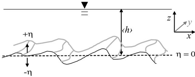
**Figure 3.** Definition sketch of the model shown in oblique perspective, with coordinate axes displayed. The mean elevation of the sediment-fluid interface (channel bottom) is shown by the dashed line, which is defined as  $\eta = 0$  and used as the datum for mean water depth,  $\langle h \rangle$ . Elevations above and below this line are positive and negative, respectively.
