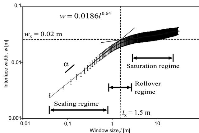
**Figure 2.** Example of North Loup River spatial scaling of roughness for 20 downstream profiles, averaged at a snapshot in time. Interface width grows as a power law in the scaling regime, with the slope equal to the roughness exponent  $\alpha$ ; equation is a best fit linear regression to log-log data. Growth rolls over at the transition length  $l_x$ , with corresponding roughness value,  $w_x$ . Error bars represent one standard deviation.
