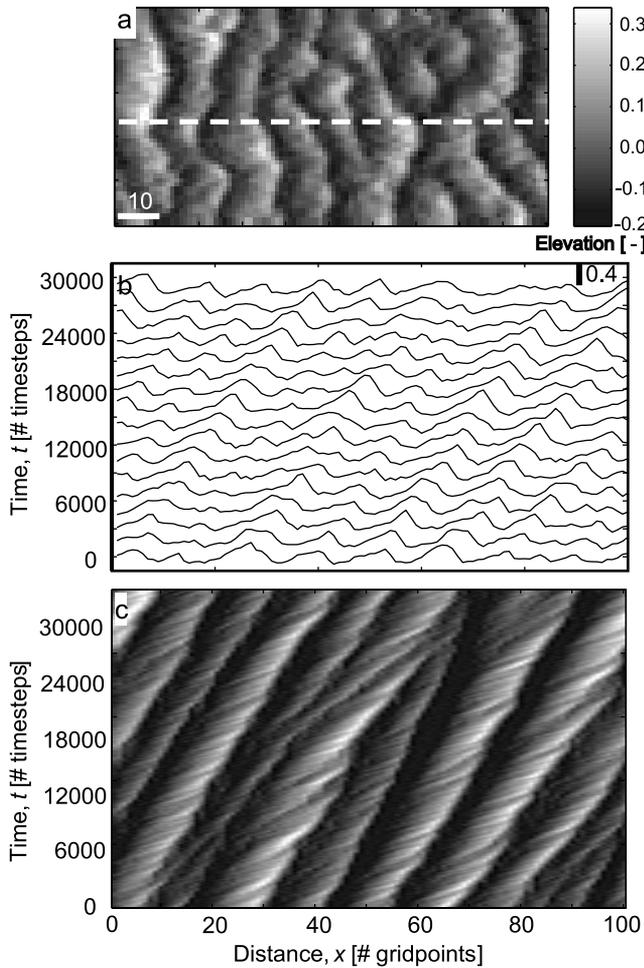
**Figure 6.** Stochastic model topography (run S, Table 1) where roughness is in statistical steady state; compare to Figure 1. (a) Plan view snapshot. (b) Sequential profiles shown every  $1500\Delta t$ . (c) Space-time plot of sequential profiles shown every time step.
