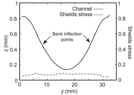
FIG. 4. An example profile of the channel geometry, with  $y$  as the cross-stream and  $z$  as the vertical coordinates, together with the Shields stress profile. The profiles are the average of all  $\sim 100$  of the cross-stream profiles of Shields stress and channel geometry for this given width within a scan. The widths averaged fell within the range of an individual pixel's width of 0.93 mm.
