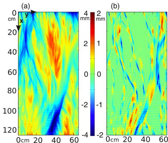
FIG. 2. (Color online) (a) A scan of the topography of the braided river, with flow in the  $x$  direction from top to bottom of the image. (b) The differenced topography between the scan in (a) and the scan taken 5 min later, giving a map of the erosion and deposition that has occurred in the interval.
