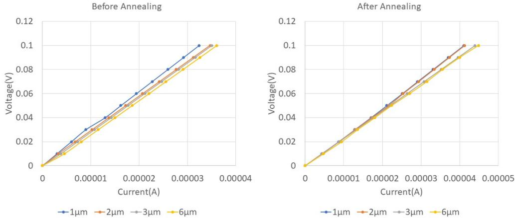
FIG. 5. Voltage versus current characteristics for contacts of radius  $1\mu\text{m}$ ,  $2\mu\text{m}$ ,  $3\mu\text{m}$  and  $6\mu\text{m}$
