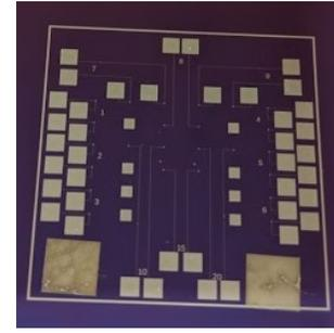
FIG. 4. 26mm x 26mm Contact resistance measurement device
