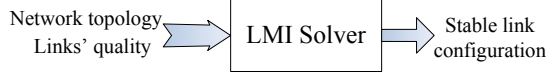
Figure 3. A procedure used to extract a stabilizing configuration for the Wireless Control Network.
