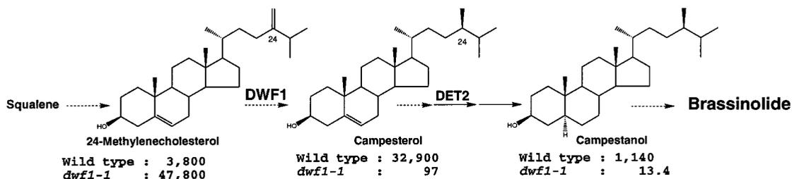
**Figure 4.** Brassinosteroid-biosynthetic step found to be defective in *dwf1* plants. The aerial parts of 5-week-old wild-type and *dwf1* plants were subjected to analysis of endogenous brassinosteroid levels using GC-SIM. Accumulation of 24-methylenecholesterol with a simultaneous reduction in the campesterol level suggests that a specific step, C-24 reduction, was blocked in *dwf1* mutants. Campesterol is known to serve as substrate for brassinolide biosynthesis.
