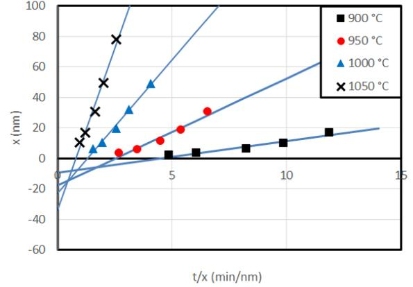
FIG. 2. A plot of  $x$  vs  $t/x$ . The black squares, red circles, blue triangles, and crosses show the measured thicknesses processed at 900, 950, 1000, and 1050 °C, respectively. The solid blue lines are the linear trend lines. The native oxide thickness of 1.3 nm is subtracted from the measured thicknesses. The intercept at  $t/x = 0$  indicates  $-A$ , and the slope gives  $B$  in Eq. (7).
